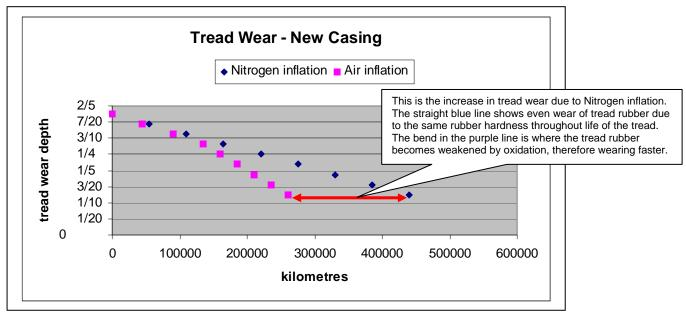
average per Goodyear), a tread wear penalty due to uneven tread contact, and a casing life penalty due to hotter casing running temperatures.
