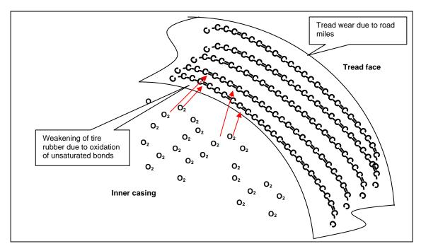
the casing, and closer towards the outside of the tire, including the tread face. At some stage the two surfaces meet. The outer tread wear face comes into contact with the degraded rubber layer. At this point, the durometer hardness of the rubber changes, and typically tread wear accelerates. The remainder of the tread wears at a much faster rate than the new tread did. This phenomenon is shown in the following chart.
