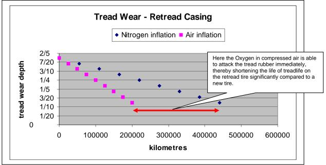
wear of the retread is the same as it is for nitrogen-inflated new casings. This means that fleets should incorporate nitrogen inflation in their entire fleet (new tires, new retreads, and old retreads) all at once. Once retreads start to be put on new tires that started their life cycle with nitrogen inflation, then not only will tread wear be longer, but the casings will be much stronger, and failures on the road will be dramatically reduced.
